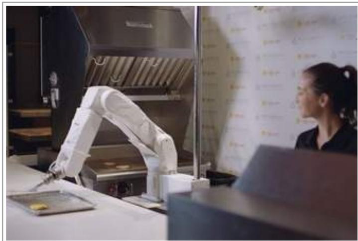
Miso Robotics created Flippy, an autonomous robotic arm that can flip burgers. A restaurant in Pasadena, Calif. has installed one to cook its meat. [Miso Robotics]
